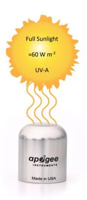
Example of UV-A measurement with an Apogee UV-A sensor. Full sunlight yields UV-A radiation on a horizontal plane at the Earth's surface of approximately 60 W m $^{-2}$ . This yields an output signal of 6 mV. The signal is converted to UV-A radiation by multiplying by the calibration factor of 10 W m $^{-2}$  per mV.
